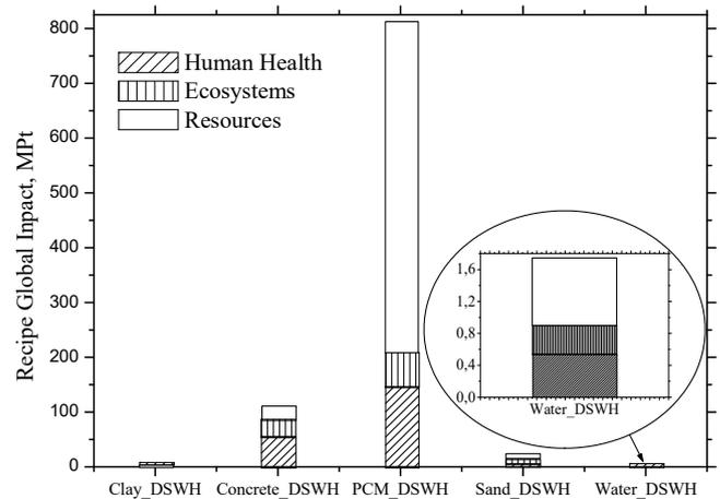
**Fig 4.** Global impact of each storage materials for solar water heater
