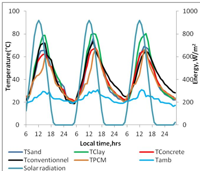
**Fig3:** Variation of the incident solar flux, the ambient temperature and the water outlet temperature according to the local time during two successive days (06-08/06).
