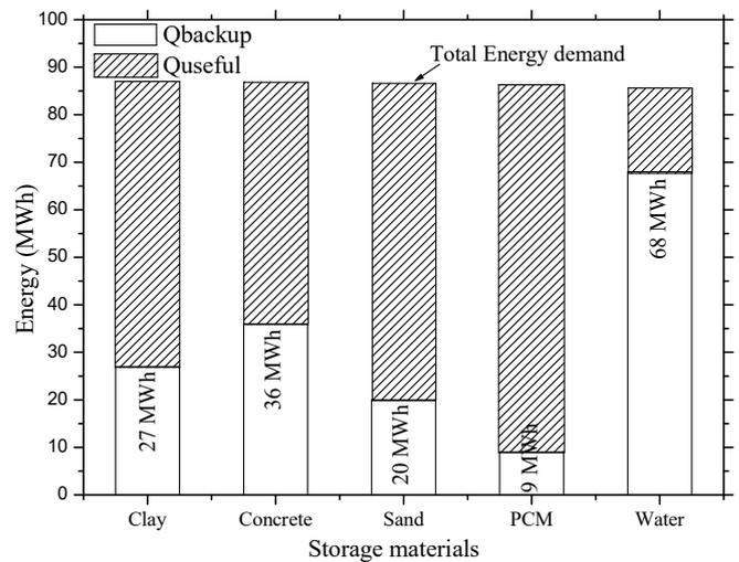
**Fig 4:** Comparative study for thermal storage materials energetic performance during their lifespan (20 years).
